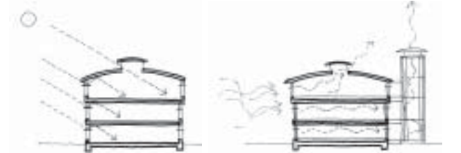
Daylight Penetration Light shelves and roof monitors allow daylight to reach every workspace.
